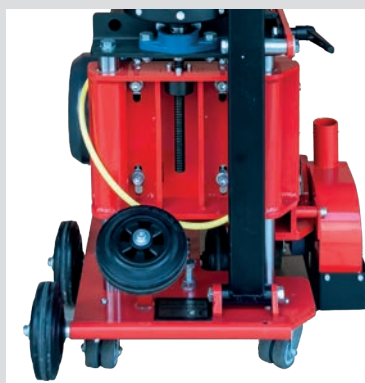
Removable wheel for corner milling
