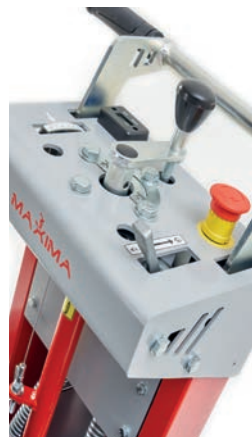
Adjustable depth and accelerator with "neutral" lock
