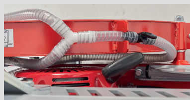
Double water inlet for improved blade cooling
