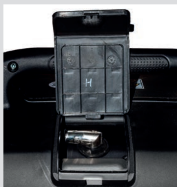
Easy access for spark plug maintenance
