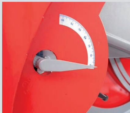
Cutting depth indicator
