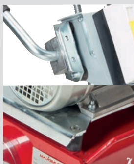
Dual grip and motor vibration damping system
