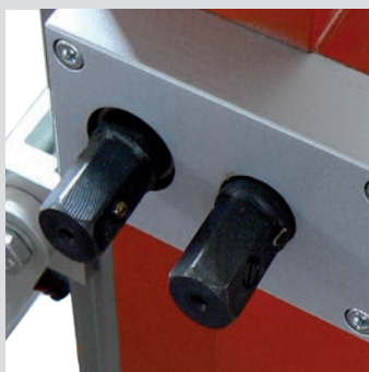
Dual speed motor carriage feed system
