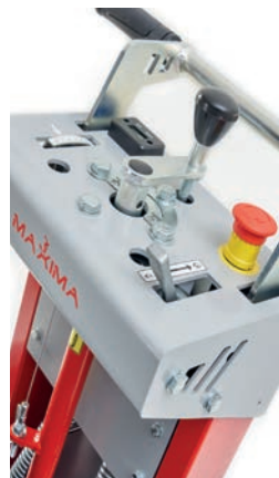
Adjustable depth and accelerator with "neutral" lock
