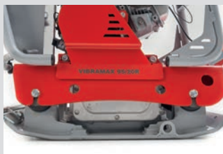
Vibration-damping rubber on the base
