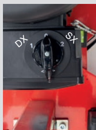
Switch with direction inverter
