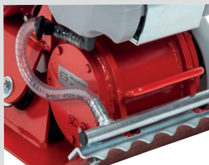
Bumper bar and knurling for drip tray
