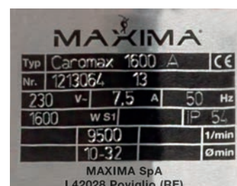
High speed motor: 9500 rpm
