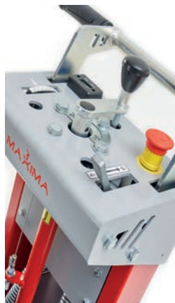
Adjustable depth and accelerator with "neutral" lock
