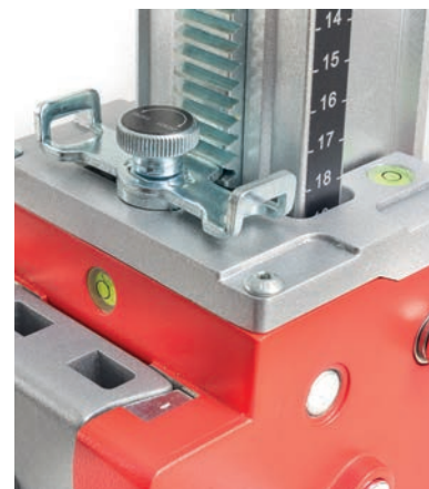
Double spirit level and lowering stop lever
