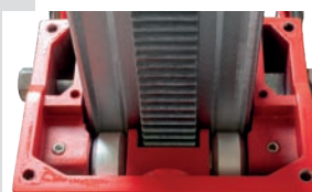
Sliding on shielded bearings
