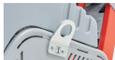
Double lifting hook
