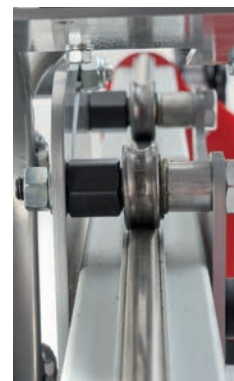
Steel bearings sliding in two double steel bars
