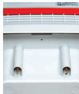
Water sensors under the motor
