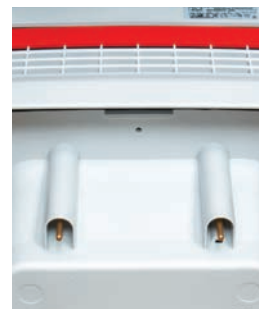
Water sensors under the motor
