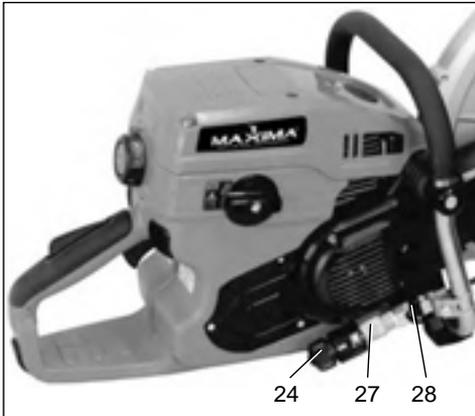
Fine dust occurs when cutting mineral materials. Recommendation: Use the water connection and cut-off wheels suitable for wet cutting when cutting mineral materials.
