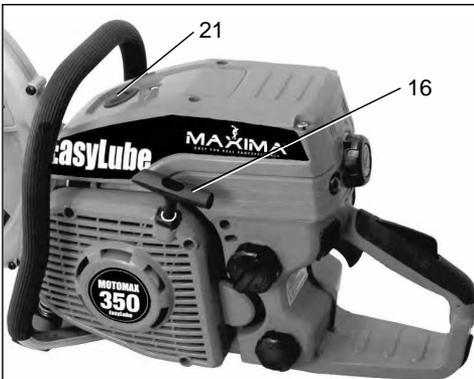
When the decompression valve (21) is depressed, the compression pressure in the combustion chamber is reduced. This means that the engine offers less resistance during start-up, which makes it noticeably easier to start the engine.
